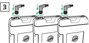
Ensure batteries are properly secured to the vessel using installed clamping brackets or tie-downs. Connect the battery terminal connectors. Push down and twist the connector collar as it is engaged. There will be an audible click to indicate connection.
