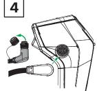
For tiller models, ensure the battery cable on the outboard is connected and locked. Fully engage the cable connector into the socket and twist-lock the connector collar fully.
