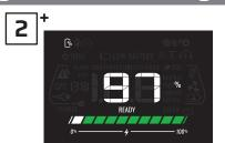
The combined state of charge (SOC) of the Avator outboard battery/batteries is shown on the display screen.
